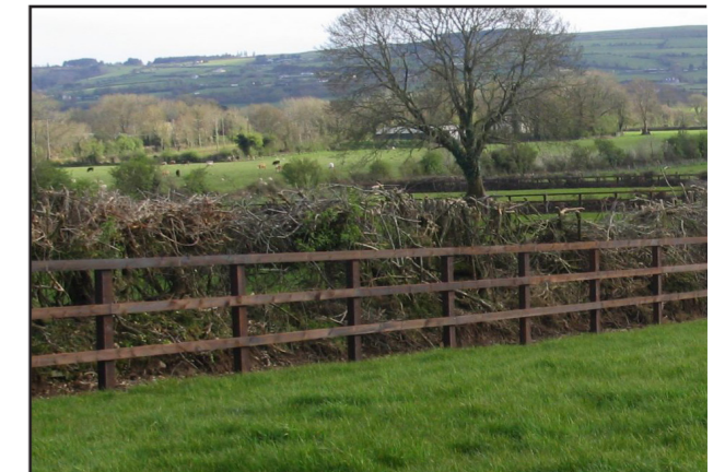
Timber Post and Rail Fence 1.4m high
